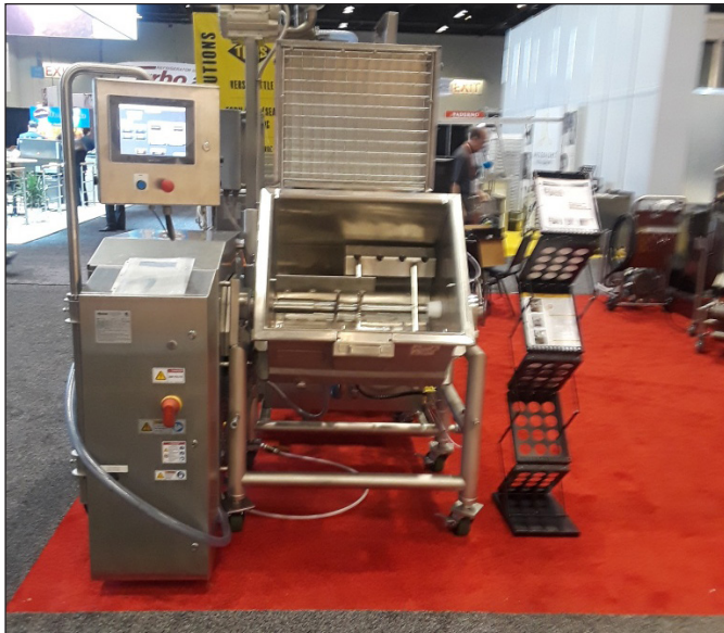
50-Gallon Gas Tilting Cooking Vessel
