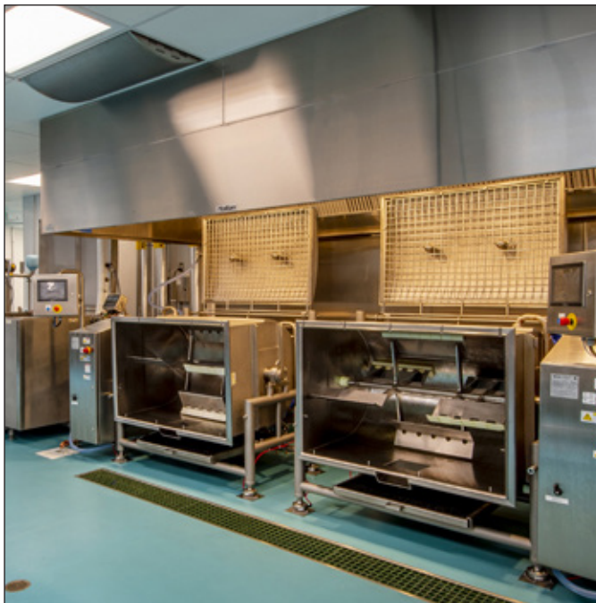
Two, 200-Gallon Tilting Versa Vessels tilted forward for agitator removal and easy cleaning
